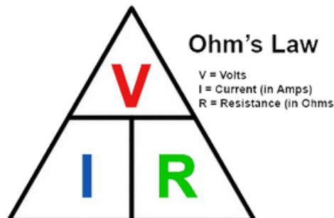
$$\frac{V}{I} = R \quad V = I \cdot R \quad (\text{volts} = \text{amps times ohms})$$
